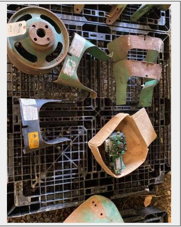
**Description** Oliver parts (four PTO shields, diesel injector pump, and belt pulley) Injector pump (condition unknown).
